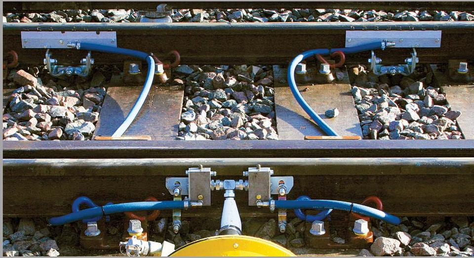
Distribution blades can be supplied in various lengths and the modular design enables easy installation and replacement with minimal blocking. There is simple blade height adjustment for precise delivery of grease to wheel flange and optional blade troughs to collect excess grease for easy cleaning. Blades can be fitted for high rail lubrication, check rail lubrication or both rails for reverse curve lubrication from one unit.
